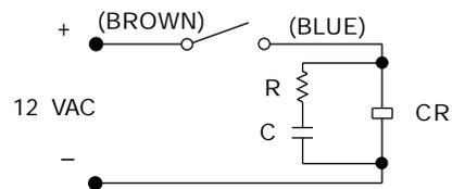
CR: Relay coil (under 2W coil rating)
