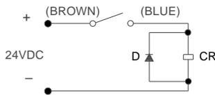
Put a resistor and capacitor in parallel with the load (CR). Select the resistor and capacitor according to the load.
