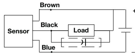
\* When connecting an inductive load (relay, solenoid valve, etc.), a protection circuit is recommended. Use a 100V, 1A diode. (NPN connection shown.)
