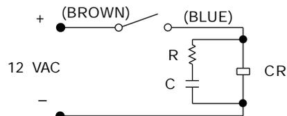
CR: Relay coil (under 2 W coil ratings)
