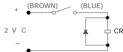
D: Diode: select a Diode with the breakdown voltage and current rating according to the load.
